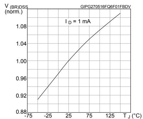
Figure 10. Normalized V_{(BR)DSS} vs temperature
